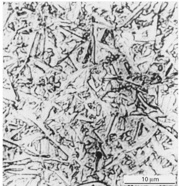
Figure 7 Optical micrograph of an as-electrodeposited cobalt foil obtained at pH 2. Section parallel to the substrate.
