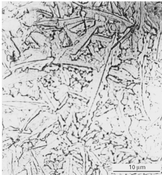
Figure 8 Optical micrograph of a cobalt deposit obtained at pH 2 and annealed 1 h at 600 °C. Section parallel to the substrate.
