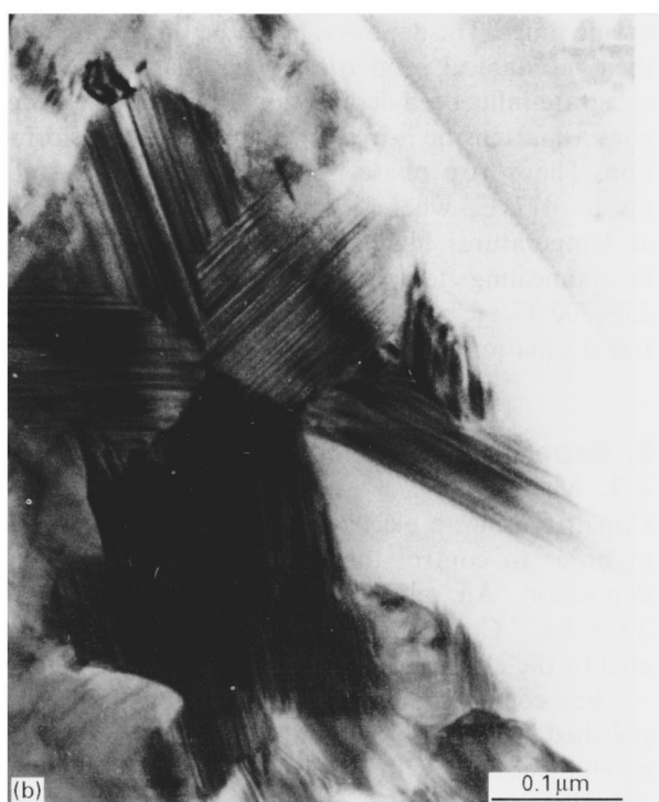
Figure 1 Transmission electron micrograph of as-electrodeposited cobalt specimens. Sections parallel to the substrate: (a) deposit obtained at pH 4, (b) deposit obtained at pH 1.5.
