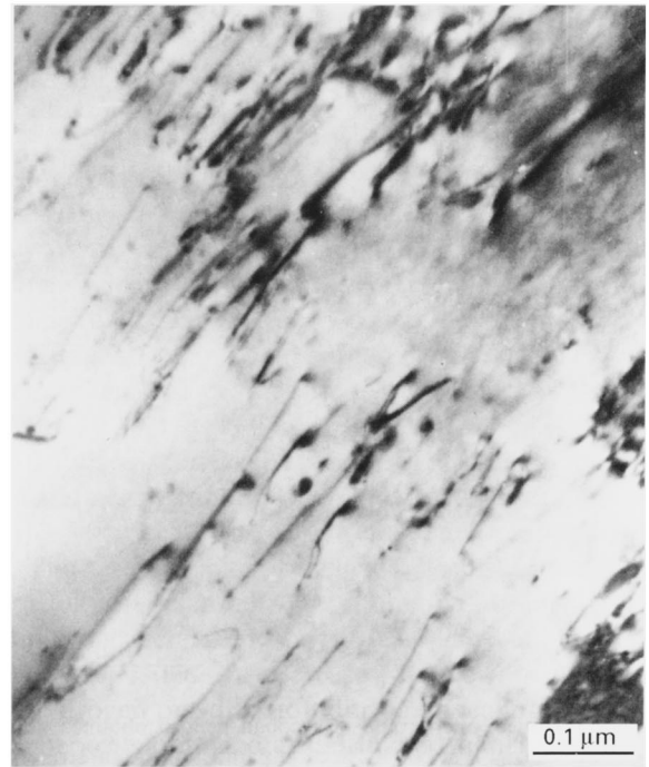
Figure 6 Transmission electron micrograph of a deposit obtained at pH 5 and annealed 1 h at 400 °C. Section parallel to the substrate.
