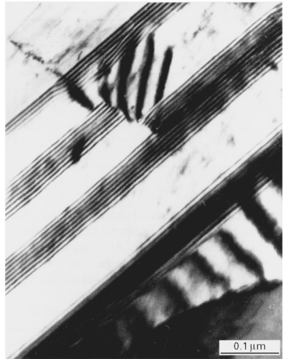
Figure 9 Transmission electron micrograph of a deposit obtained at pH 4 and annealed 1 h at 500 °C. Section parallel to the substrate.
